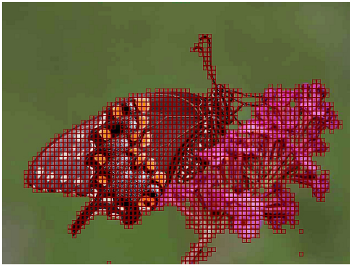
Fig. 3. Classification of regions based on local entropy. The superimposed squares indicate regions with an entropy value higher than a threshold.
